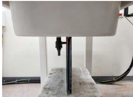
Fig.4 EUT Top side to flat phantom
