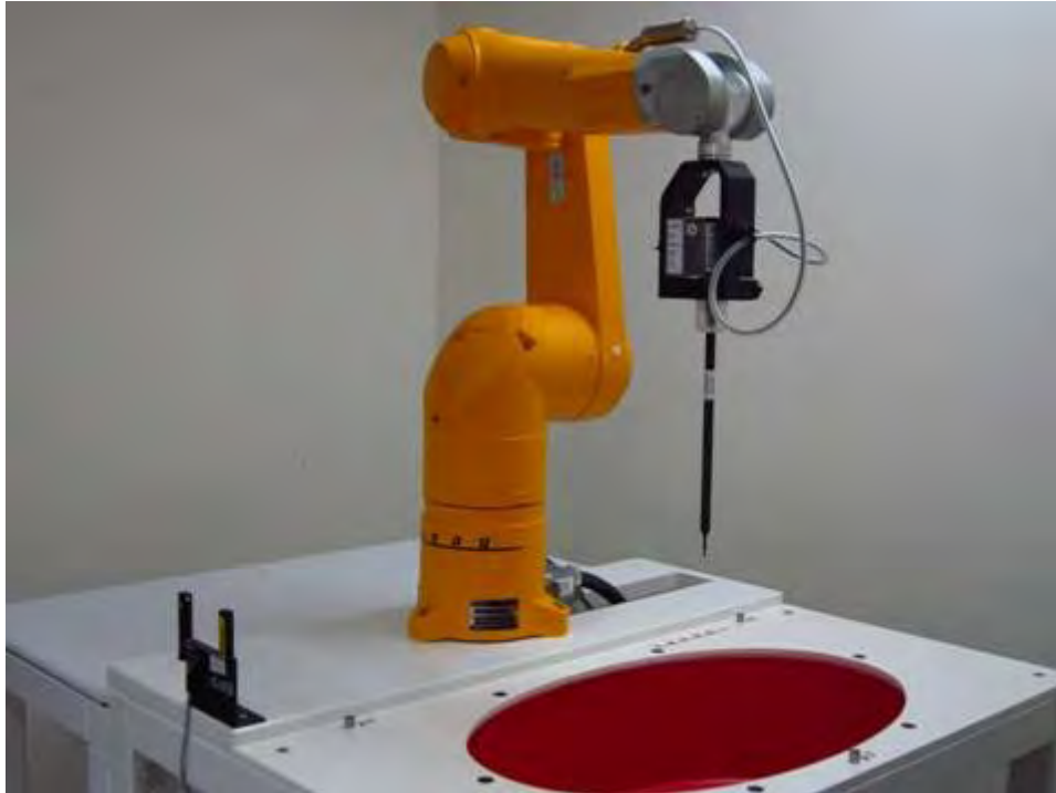
Fig.1 Photograph of the SAR measurement system
