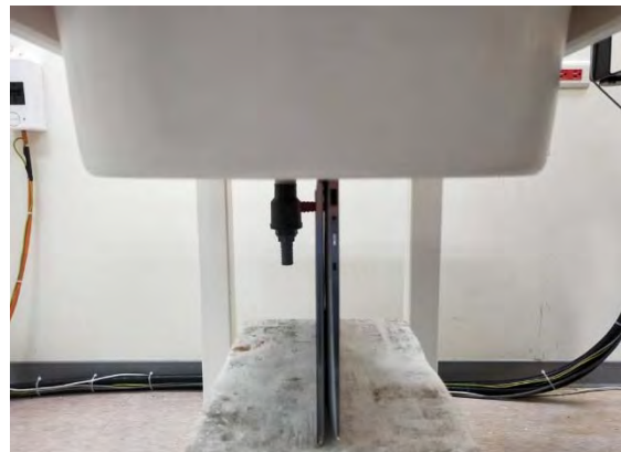
Fig.5 EUT Bottom side to flat phantom
