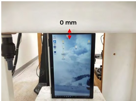
Fig.7 EUT Left side to flat phantom
