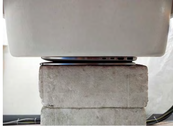
Fig.3 EUT Back side to flat phantom
