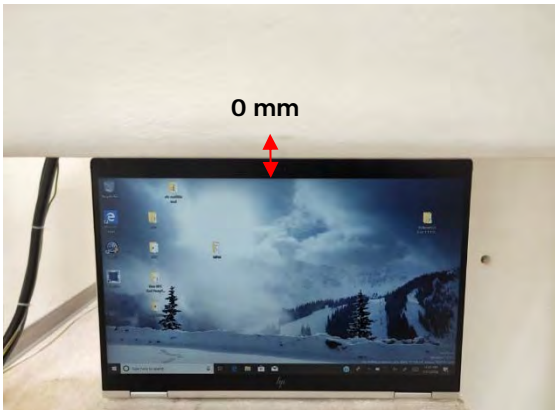
Fig.4 EUT Top side to flat phantom
