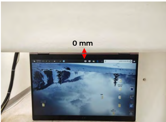
Fig.5 EUT Bottom side to flat phantom
