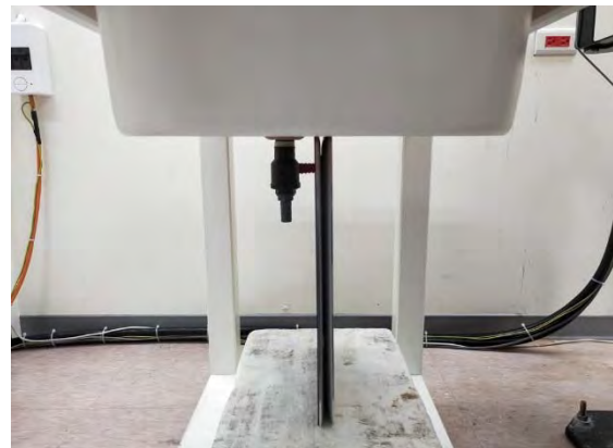
Fig.7 EUT Left side to flat phantom
