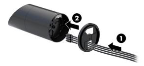
3. Hold the top piece of the mounting bracket against the bottom of the column, route the cables through the hole in the mounting surface, and then place the column over the hole on the mounting surface.
