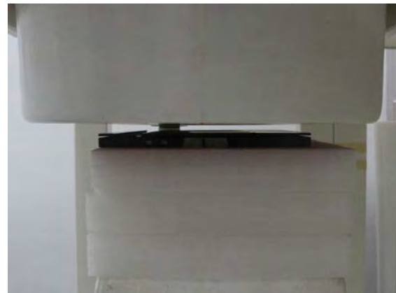
Fig.4 EUT Back side (10mm) to flat phantom
