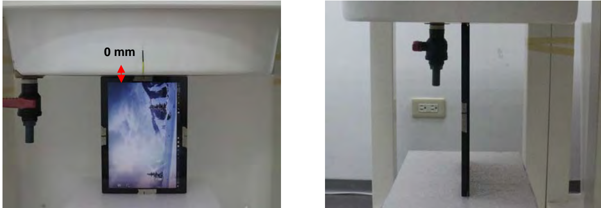
Fig.9 EUT Right side to flat phantom
