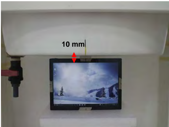
Fig.7 EUT Top side (10mm) to flat phantom
