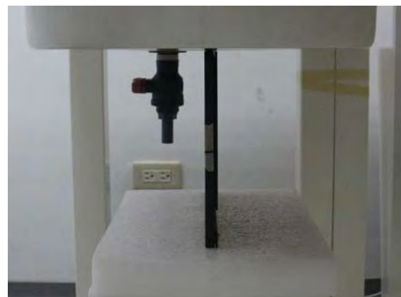
Fig.5 EUT Bottom side to flat phantom
