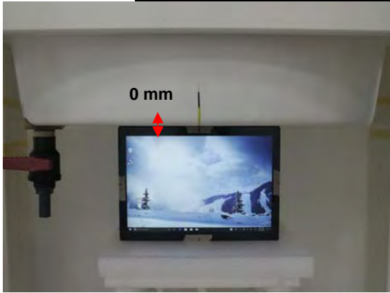
Fig.6 EUT Top side to flat phantom
