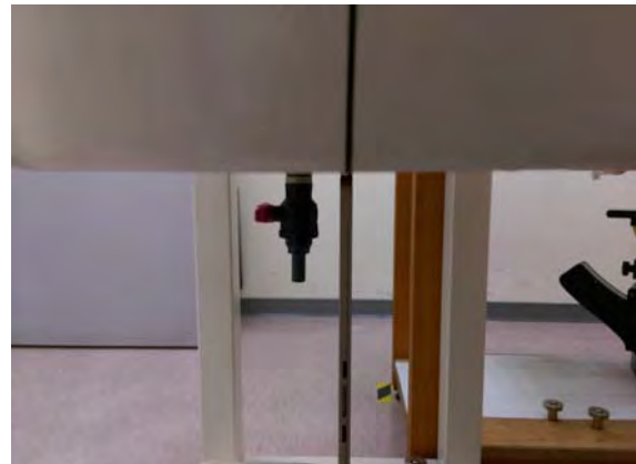
Fig.5 EUT Right side to flat phantom
