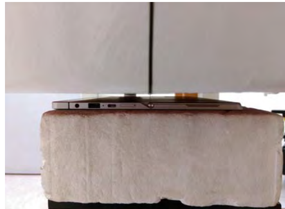
Fig.4 EUT Back side (10mm) to flat phantom
