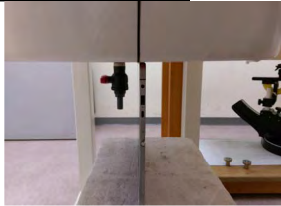
Fig.6 EUT Top side to flat phantom
