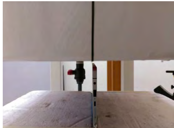
Fig.7 EUT Top side (10mm) to flat phantom
