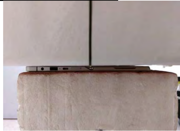
Fig.3 EUT Back side to flat phantom
