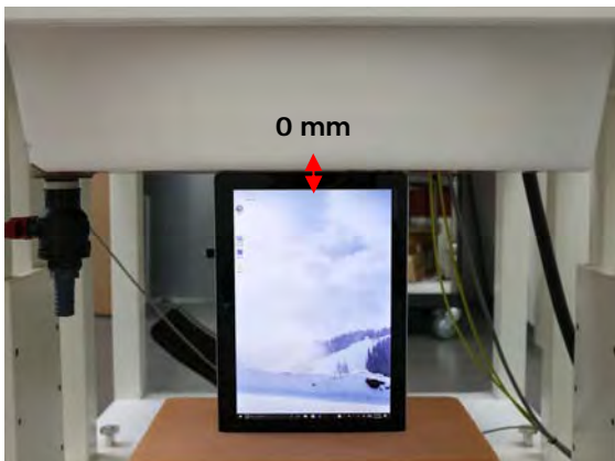
Fig.8 EUT Left side to flat phantom
