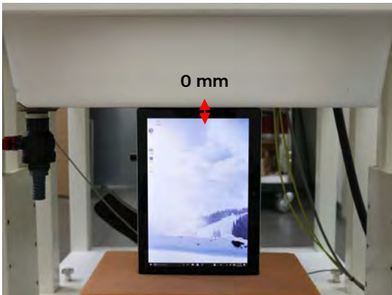
Fig.5 EUT Right side to flat phantom
