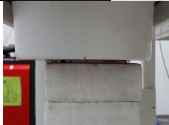
Fig.3 EUT Back side to flat phantom
