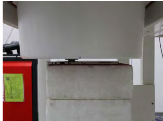
Fig.4 EUT Back side (10mm) to flat phantom
