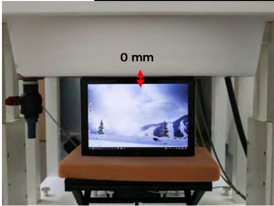
Fig.6 EUT Top side to flat phantom
