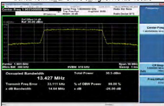
Band2 15MHz_QPSK 75 0_HighCH19125-1902.5
