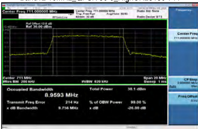
Band12 10MHz_QPSK 50 0_HighCH23130-711
