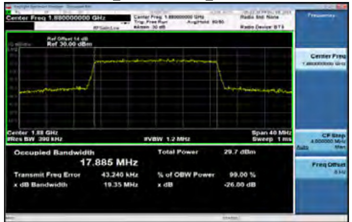
Band2 20MHz_16-QAM 100 0_MidCH18900-1880
