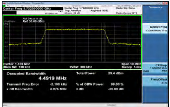
Band4 5MHz_16-QAM 25 0_MidCH20175-1732.5
