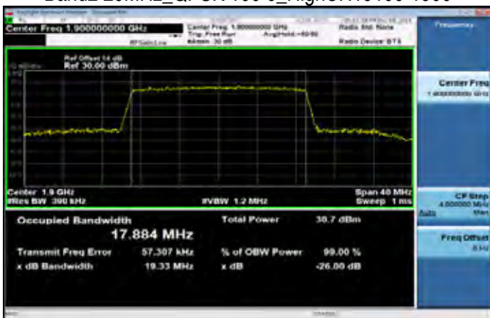
Band2 20MHz_QPSK 100 0_HighCH19100-1900
