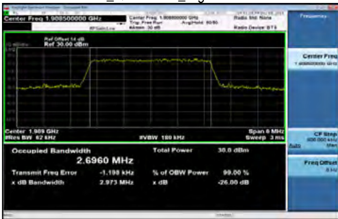
Band2 3MHz_QPSK 15 0_HighCH19185-1908.5
