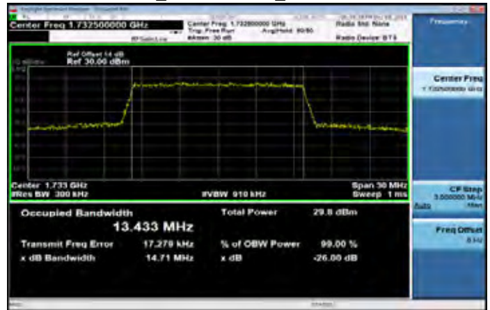
Band4 15MHz_16-QAM 75 0_MidCH20175-1732.5
