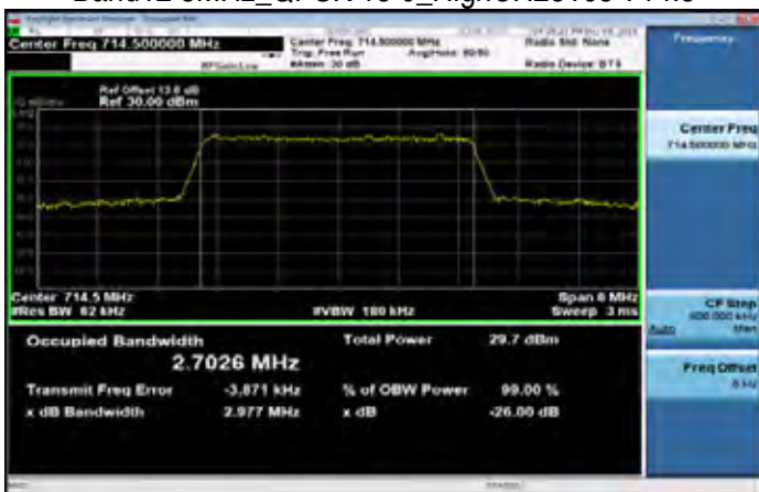
Band12 3MHz_QPSK 15 0_HighCH23165-714.5
