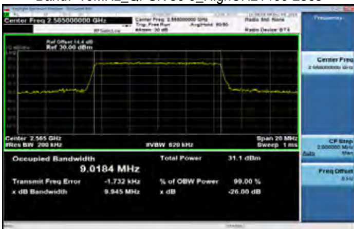
Band7 10MHz_QPSK 50_0_HighCH21400-2565
