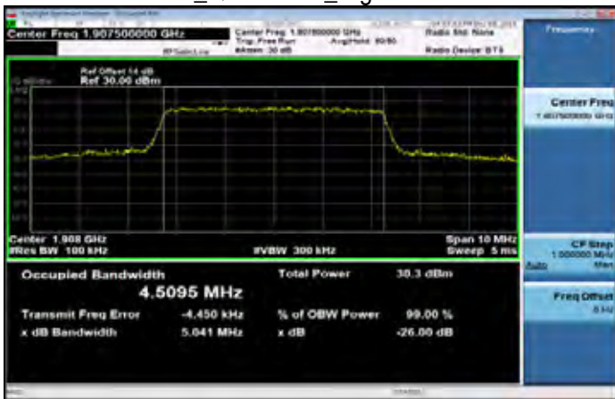
Band2 5MHz_QPSK 25 0_HighCH19175-1907.5
