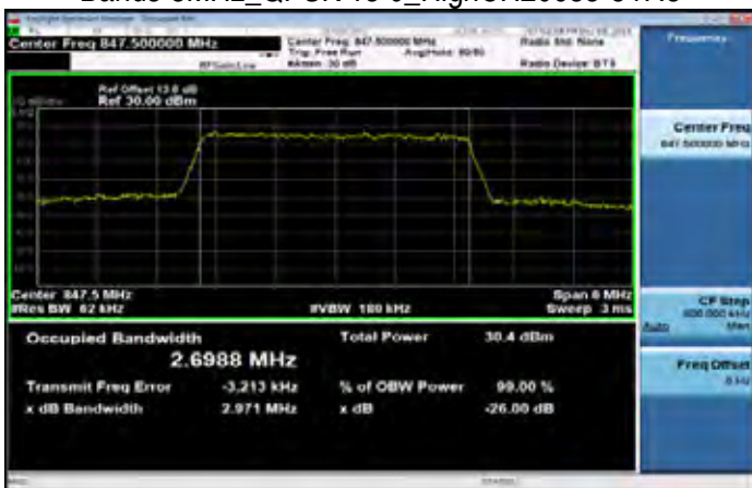
Band5 3MHz_QPSK 15 0_HighCH20635-847.5
