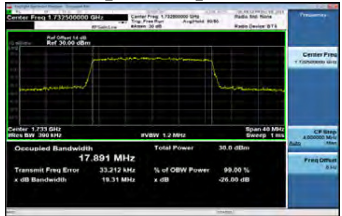
Band4 20MHz_16-QAM 100 0_MidCH20175-1732.5
