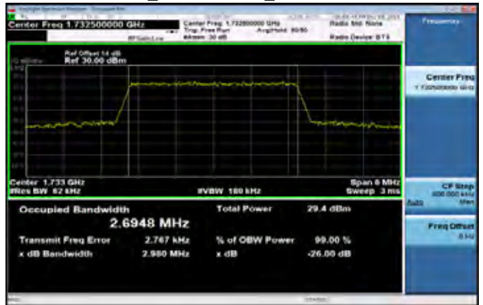
Band4 3MHz_16-QAM 15 0_MidCH20175-1732.5
