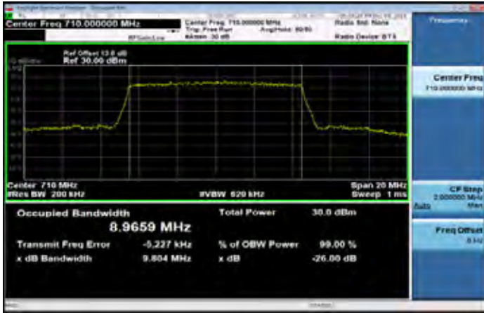
Band17 5MHz_16-QAM 25 0_MidCH23790-710
