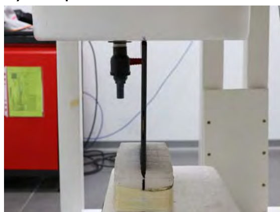
Fig.5 EUT Right side to flat phantom
