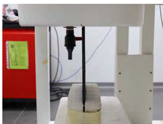
Fig.8 EUT Left side to flat phantom
