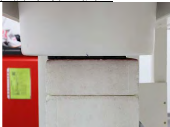
Fig.3 EUT Back side to flat phantom
