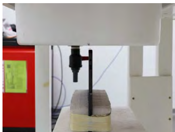
Fig.7 EUT Top side (10mm) to flat phantom
