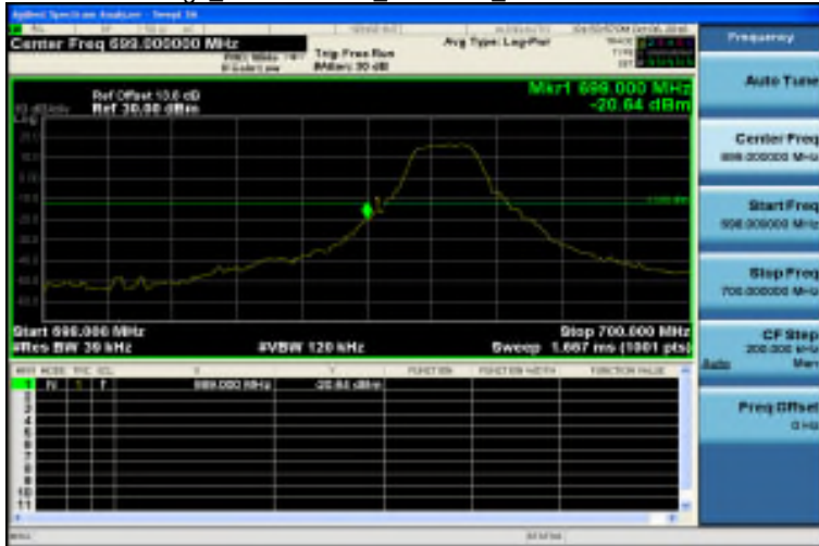
Band Edge_Band12 3MHz_QPSK 1 0_LowCH23025-700.5
