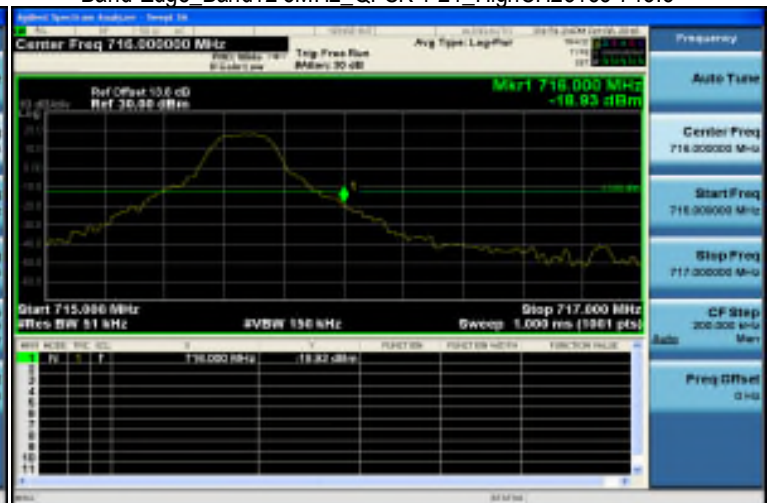
Band Edge_Band12 5MHz_QPSK 1 24_HighCH23155-713.5
