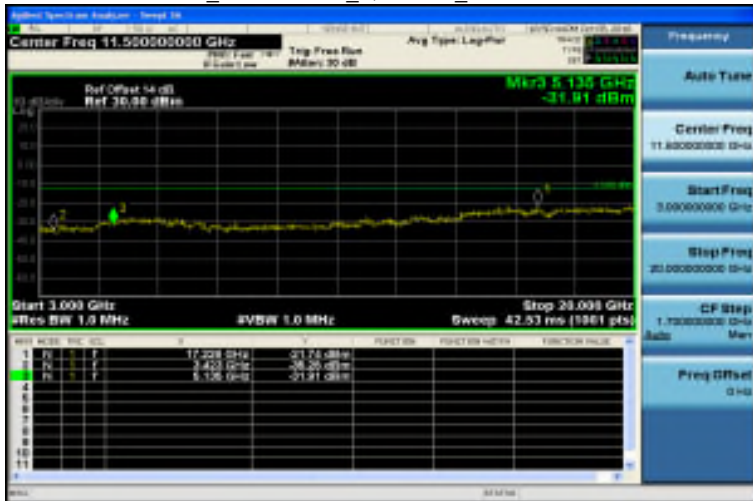
3GHz~10GHz_Band4 3MHz_QPSK 1 0_LowCH19965-1711.5
