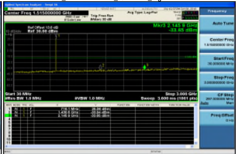
30MHz~3GHz_Band12 1.4MHz_QPSK 1 0_HighCH23173-715.3
