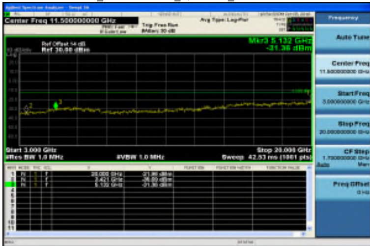
3GHz~10GHz_Band4 1.4MHz_QPSK 1 0_LowCH19957-1710.7
