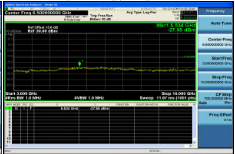
3GHz~10GHz_Band12 5MHz_QPSK 1 0_MidCH23095-707.5
