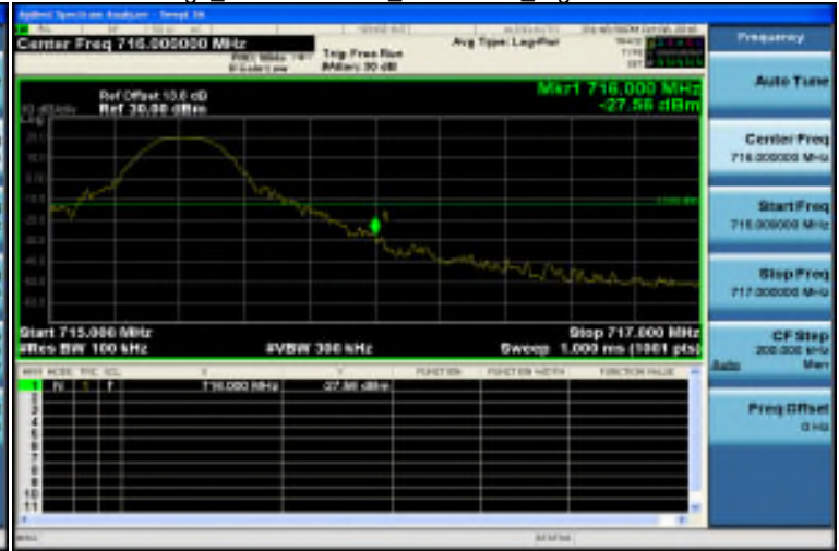
Band Edge_Band12 10MHz_QPSK 1 49_HighCH23130-711
