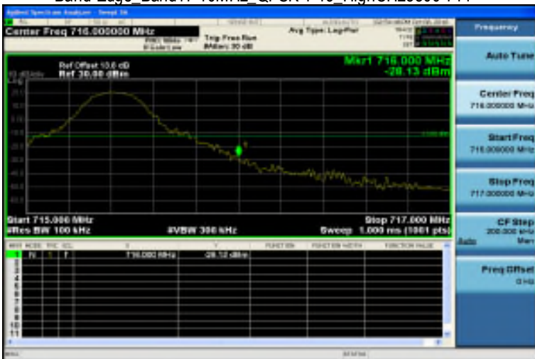
Band Edge_Band17 10MHz_QPSK 1 49_HighCH23800-711
