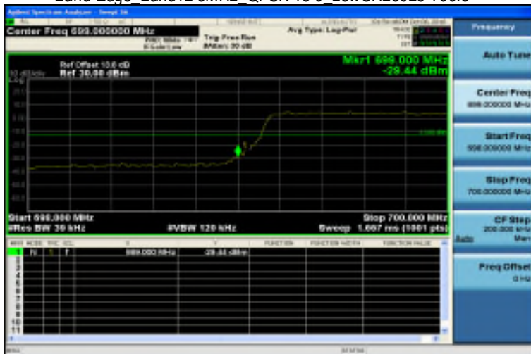
Band Edge_Band12 3MHz_QPSK 15 0_LowCH23025-700.5
