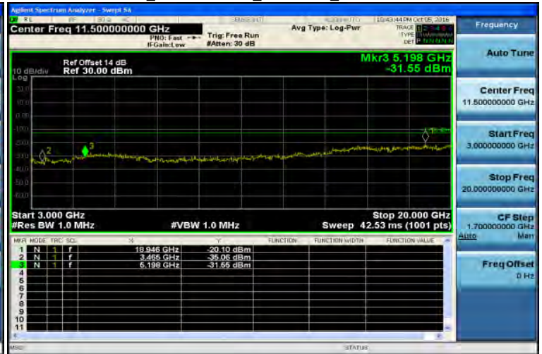
3GHz~10GHz_Band4 10MHz_QPSK 1 0_MidCH20175-1732.5
