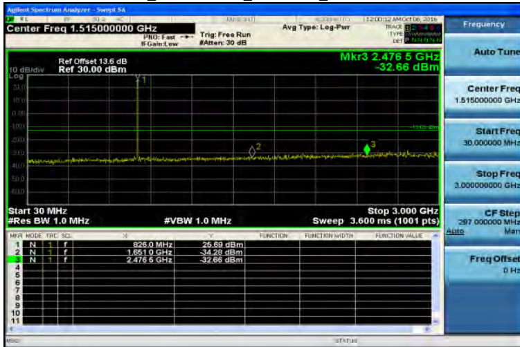
30MHz~3GHz_Band5 3MHz_QPSK 1_0_LowCH20415-825.5
