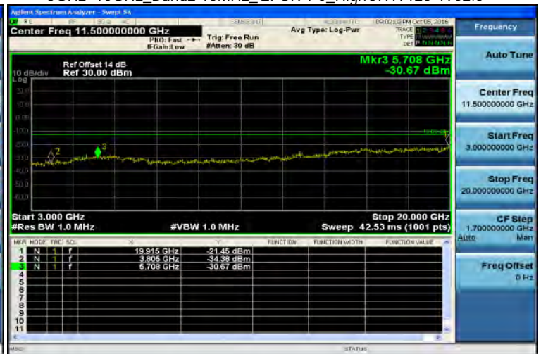
3GHz-10GHz_Band2 15MHz_QPSK 1_0_HighCH19125-1902.5
