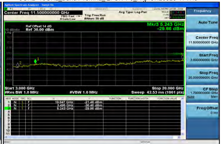
3GHz-10GHz_Band4 15MHz_QPSK 1_0_HighCH20325-1747.5
