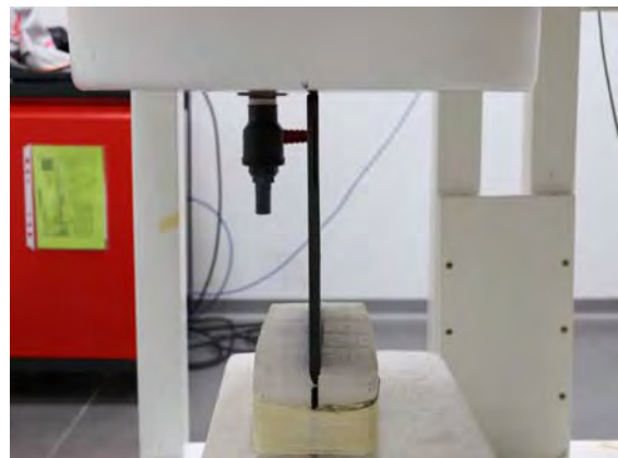
Fig.8 EUT Left side to flat phantom
