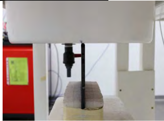
Fig.6 EUT Top side to flat phantom
