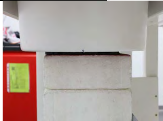
Fig.3 EUT Back side to flat phantom
