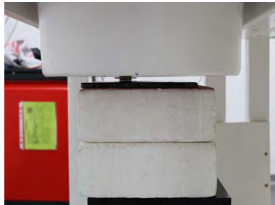
Fig.4 EUT Back side (10mm) to flat phantom
