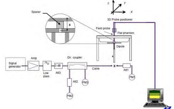
Fig. b The block diagram of system verification
