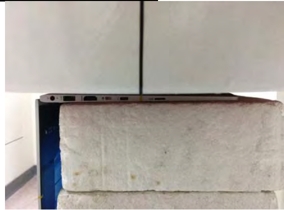
Fig.6 EUT Laptop mode to flat phantom
