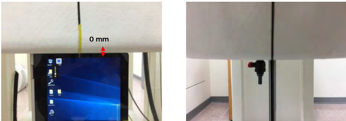
Fig.4 EUT Left side to flat phantom
