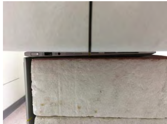
Fig.7 EUT stand mode to flat phantom
