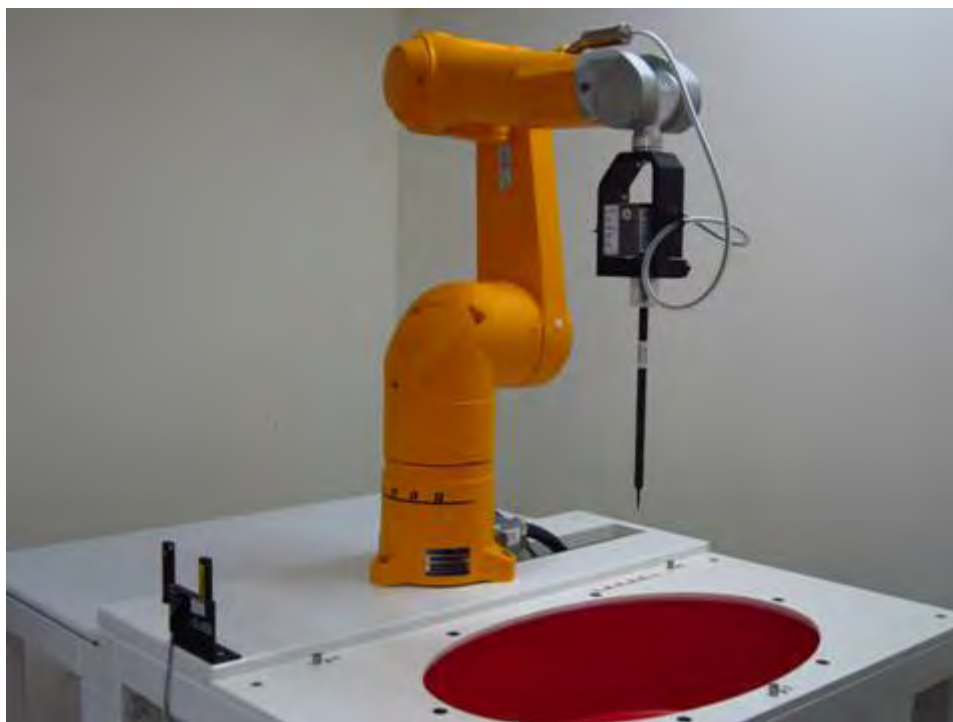
Fig.1 Photograph of the SAR measurement system
