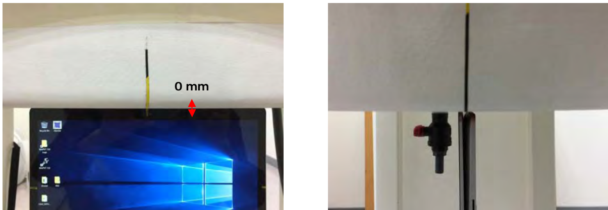
Fig.5 EUT Top side to flat phantom
