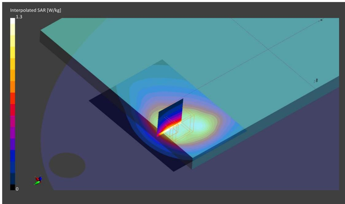
**9. LTE Band 30, QPSK - 10MHz, CH27710, Main Antenna – Back Face**
