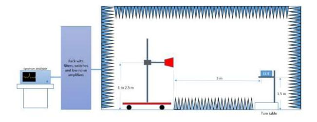
Radiated Setup 18 GHz - 26.5 GHz
