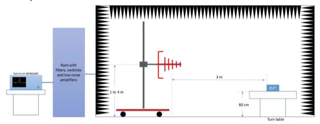
Radiated Setup 1 GHz - 18 GHz
