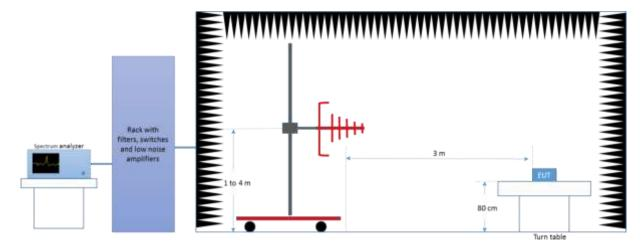
Radiated Setup 1 GHz - 18 GHz
