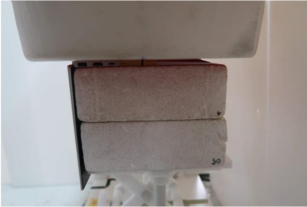
Bottom of Laptop, Test Separation 0 mm
