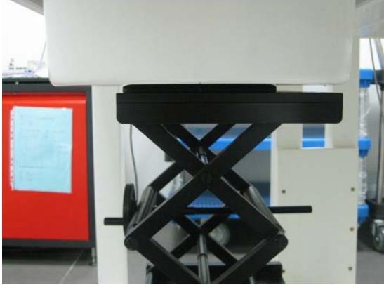
Fig.3 EUT Lap-held mode to flat phantom
