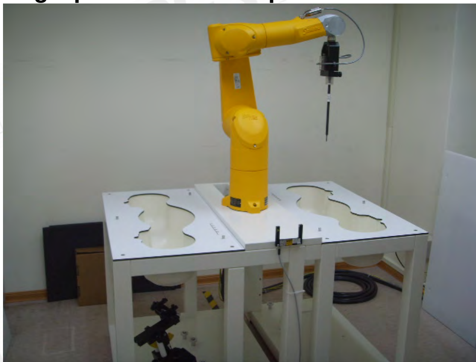
Fig.1 Photograph of the SAR measurement System
