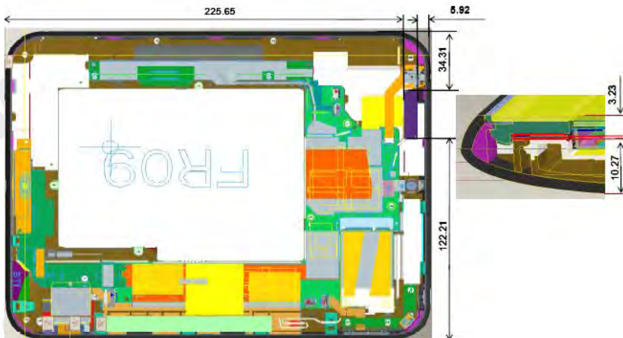
Fig.9 Antenna position &amp; distance
