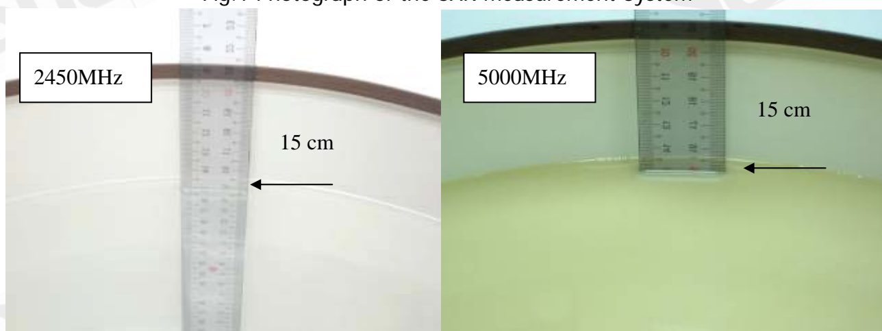
Fig.2 Photograph of the Tissue Simulant liquid depth 15cm for Flat position
