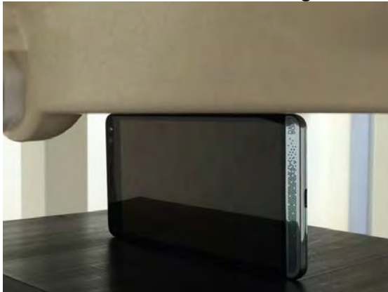
Fig.16 EUT right to flat phantom
