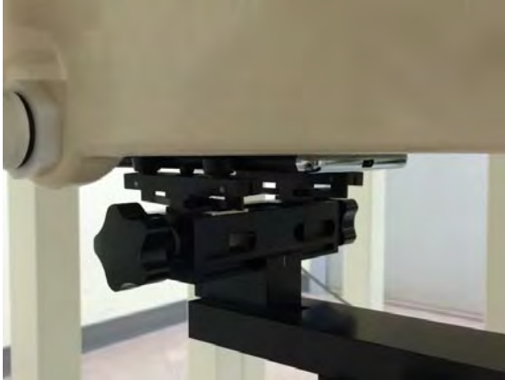
Fig.14 EUT front to flat phantom
