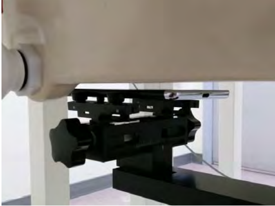
Fig.8 EUT Front side to flat phantom
