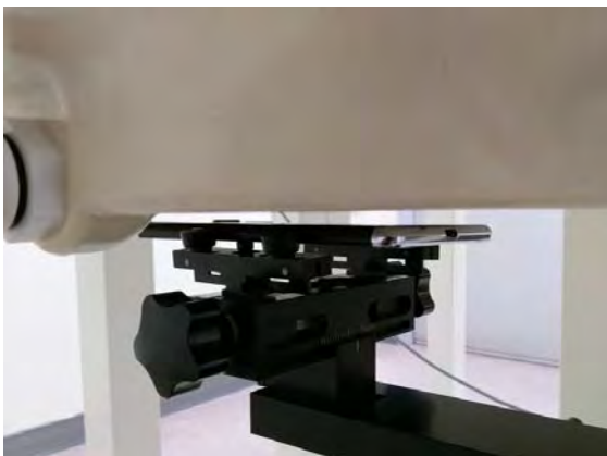
Fig.10 EUT Back side to flat phantom
