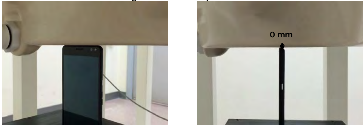
Fig.18 EUT Top side to flat phantom
