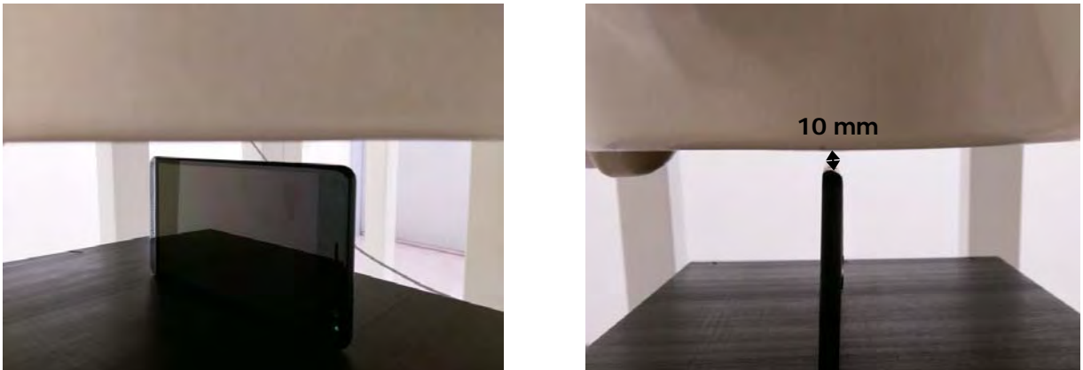
Fig.12 EUT Left side to flat phantom
