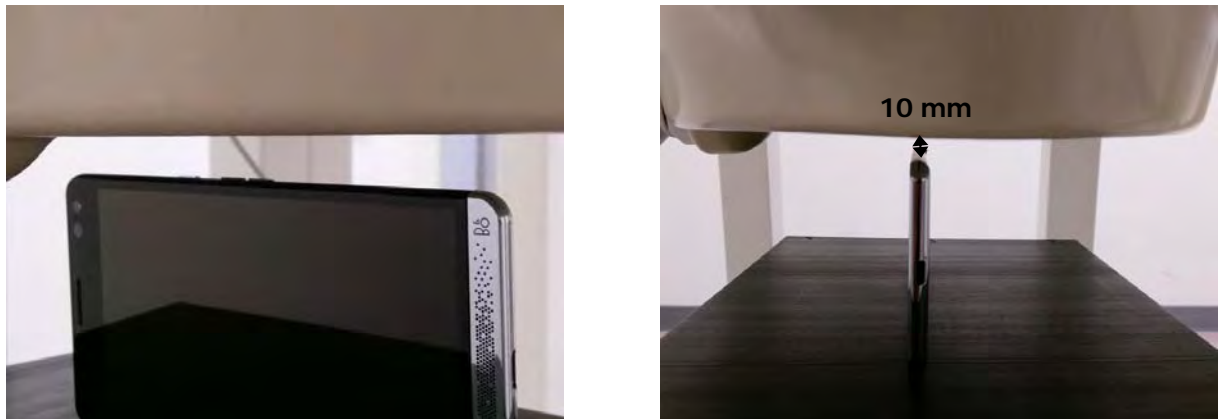
Fig.13 EUT Right side to flat phantom
