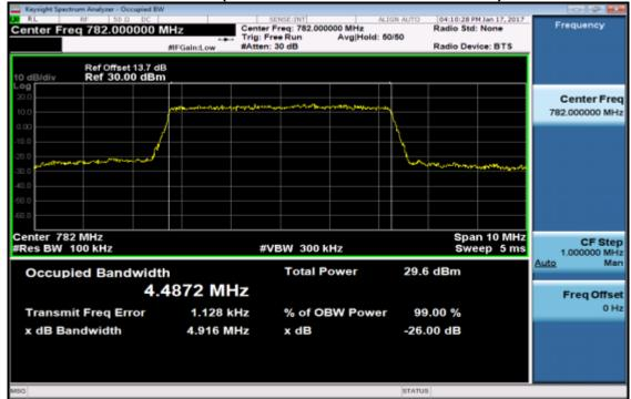
5MHz BW LTE-Band 13 (16QAM RB Number: 25 Offset: 0) Channel High
