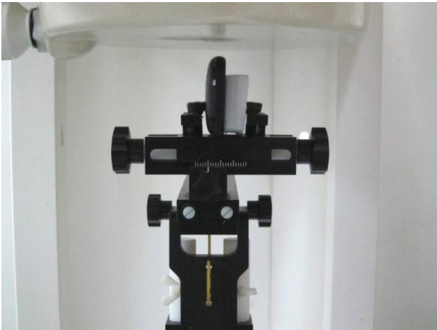
Right Side of the DUT with Phantom 1 cm Gap (DUT without Earphone)
