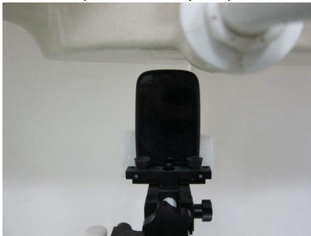
Bottom Side of the DUT with Phantom 1 cm Gap (DUT without Earphone)
