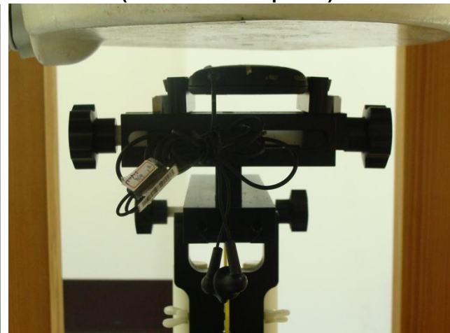
Rear Face of the DUT with Phantom 1.5 cm Gap (DUT with Earphone)
