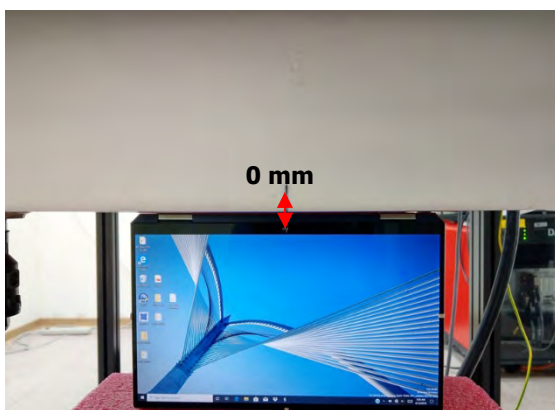
Fig.5 EUT Bottom side to flat phantom
