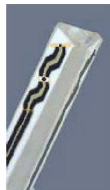
Figure 2.3 Probe Thick-Film Technique
