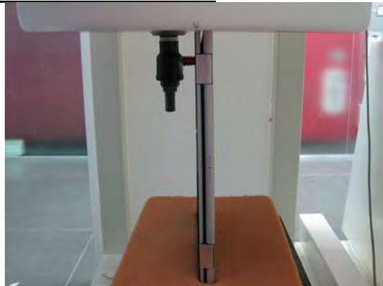
Fig.5 EUT Right side to flat phantom
