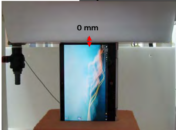
Fig.5 EUT Right side to flat phantom
