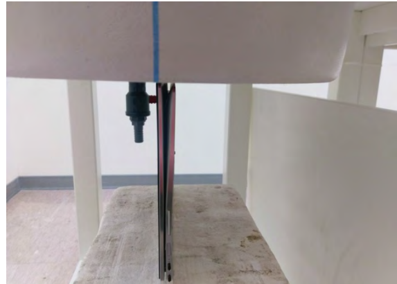
Fig.3 EUT Top side to flat phantom
