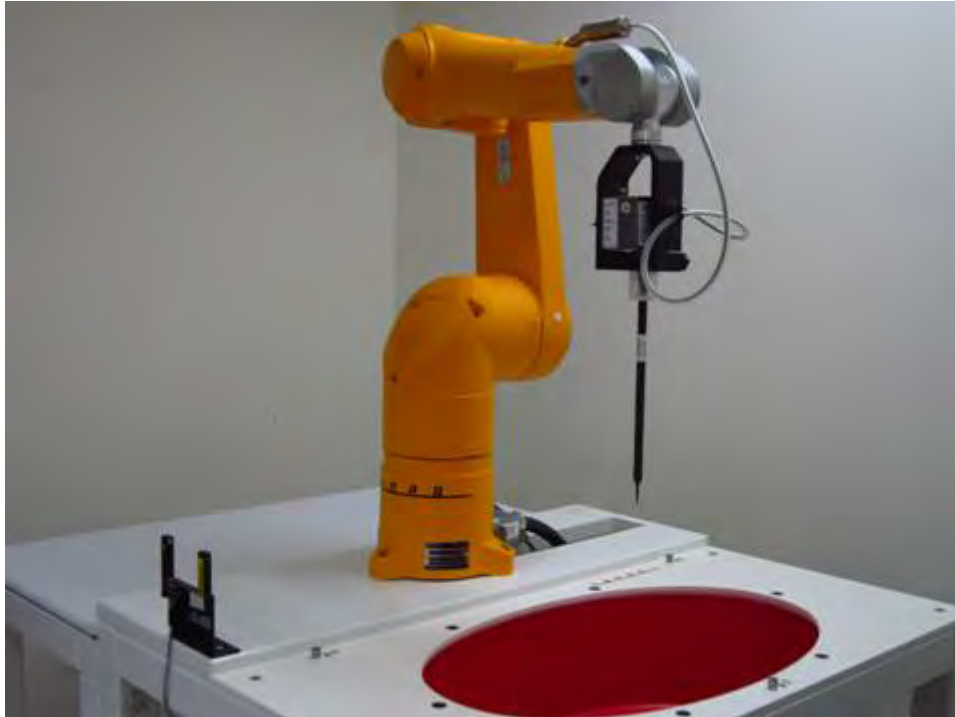
Fig.1 Photograph of the SAR measurement system
