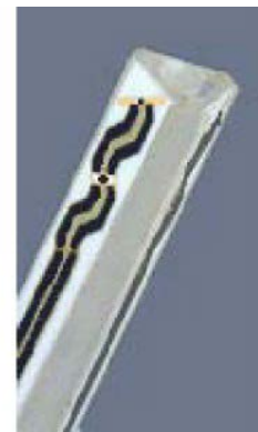
Figure 2.3 Probe Thick-Film Technique
