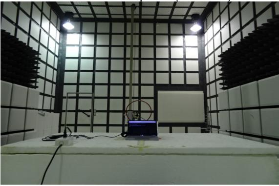
Radiated Emission Set up Photos (30MHz~1GHz)
