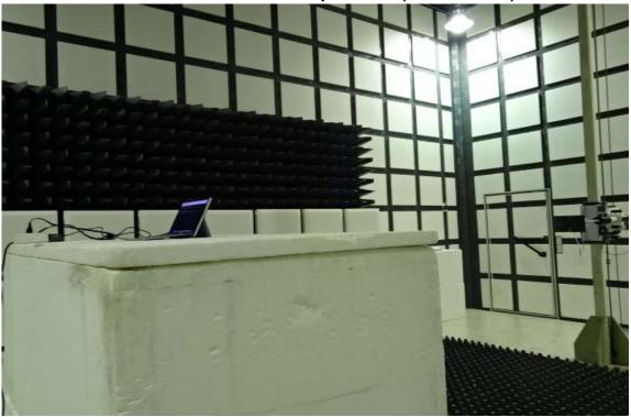
Radiated Emission Set up Photos (Front View)
