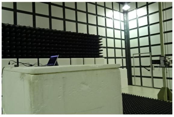
Radiated Emission Set up Photos (Front View)
