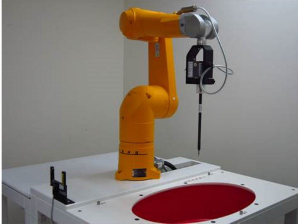
Fig.1 Photograph of the SAR measurement system
