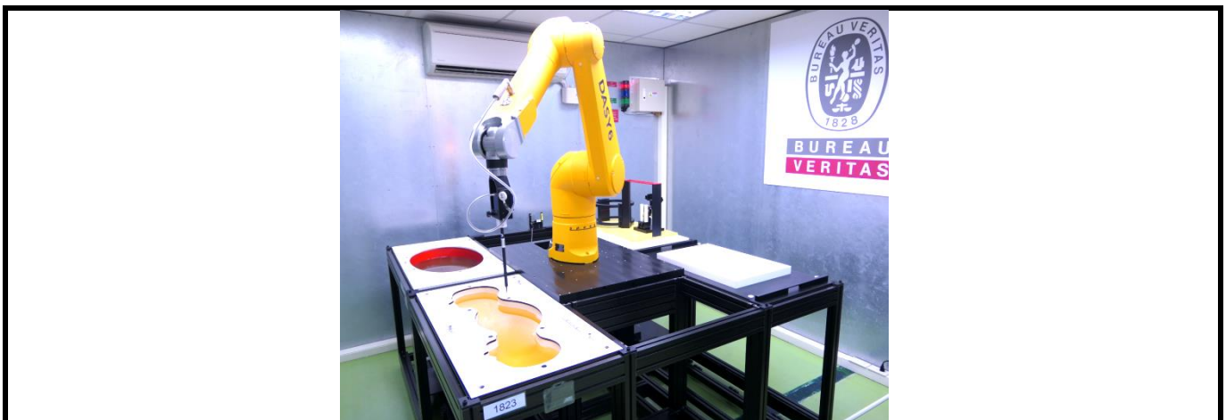
Fig-3.2 SPEAG DASY6 System
