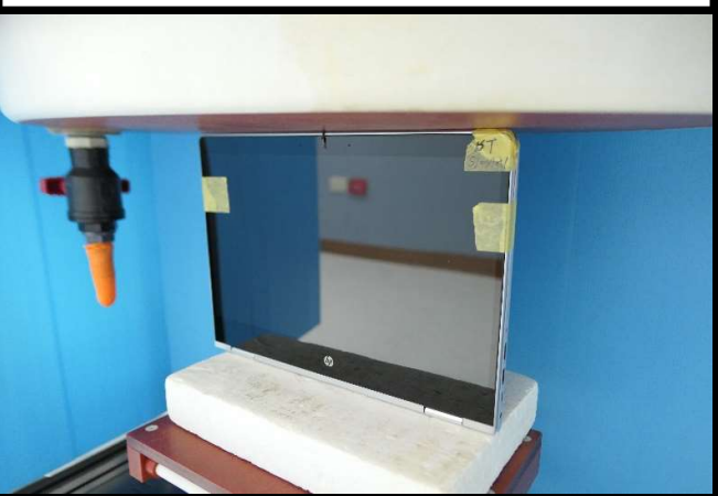
Top Side of Tablet Mode Tested at 0 mm
