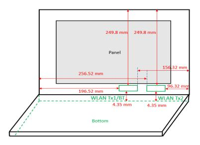
Photograph 7. Antenna position of EUT
