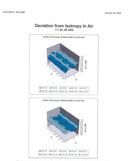
Probe isotropy for E<sub>tot</sub>: probe rotated  $\phi = 0^{\circ}$  to 360°, tilted from field propagation direction  $\vec{k}$ Parallel to the field propagation ( $\psi = 0^{\circ} - 90^{\circ}$ ) at 30 GHz: deviation within  $\pm 0.38$  dB Parallel to the field propagation ( $\psi = 0^{\circ} - 90^{\circ}$ ) at 60 GHz: deviation within  $\pm 0.33$  dB
