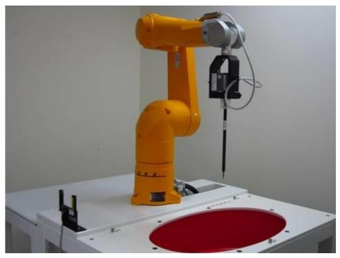
Fig.1 Photograph of the SAR measurement system
