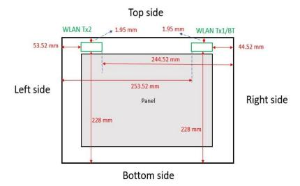
Photograph 17. Antenna position of EUT
