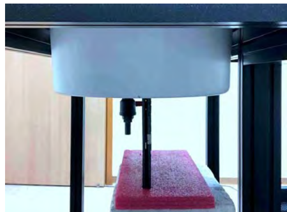
Fig.5 EUT Bottom side to flat phantom
