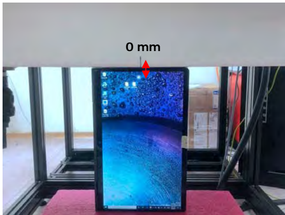
Fig.7 EUT Left side to flat phantom
