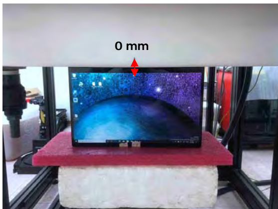
Fig.5 EUT Bottom side to flat phantom
