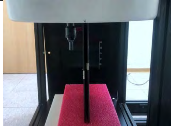
Fig.6 EUT Right side to flat phantom
