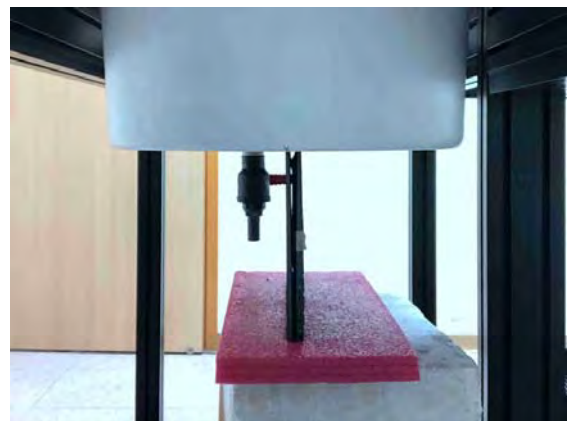
Fig.4 EUT Top side to flat phantom
