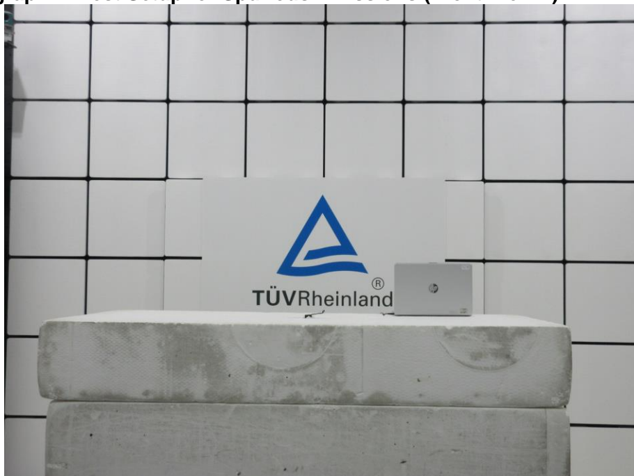
Photograph 2: Test Setup for Spurious Emissions (Front View 2)
