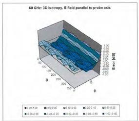
Probe isotropy for  $E_{tot}$ : probe rotated  $\varphi = 0^{\circ}$  to 360°, tilted from field propagation direction  $\vec{k}$ Parallel to the field propagation ( $\psi = 0^{\circ} - 90^{\circ}$ ) at 30 GHz: deviation within  $\pm 0.46$  dB Parallel to the field propagation ( $\psi = 0^{\circ} - 90^{\circ}$ ) at 60 GHz: deviation within  $\pm 0.44$  dB
