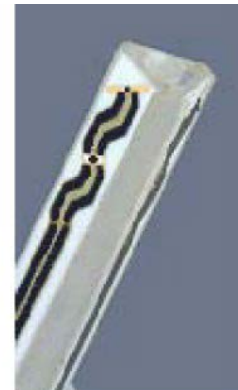
Figure 2.3 Probe Thick-Film Technique
