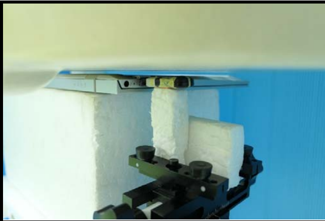
Horizontal Up of EUT Tested at 5 mm
