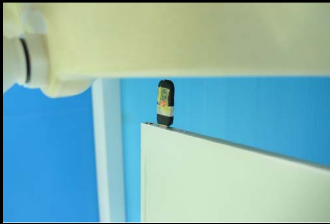
Tip Mode of EUT Tested at 5 mm
