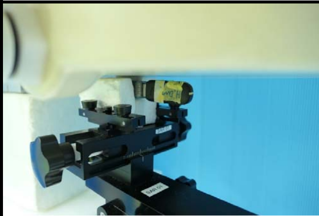
Vertical Front of EUT Tested at 5 mm
