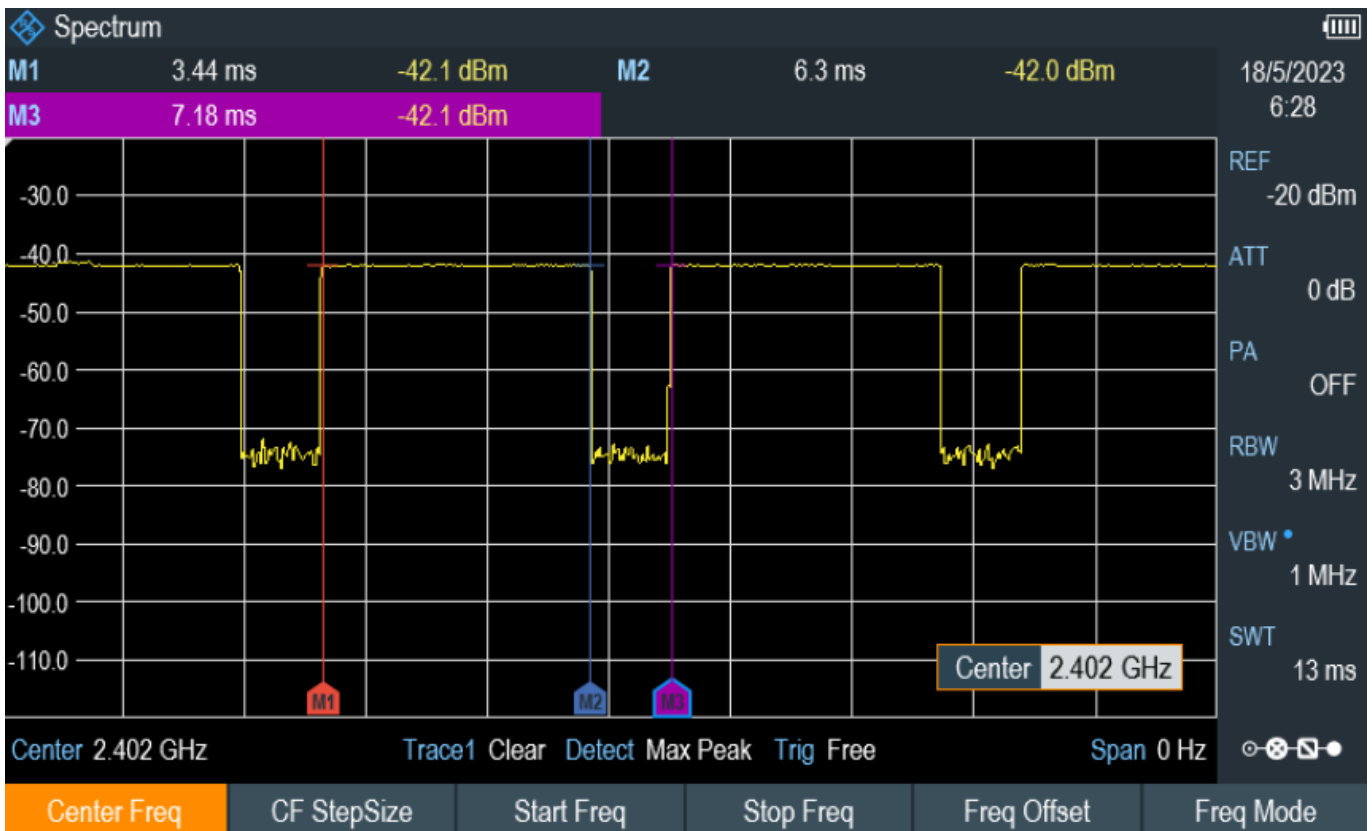
Time-domain plot for Bluetooth transmission signal
