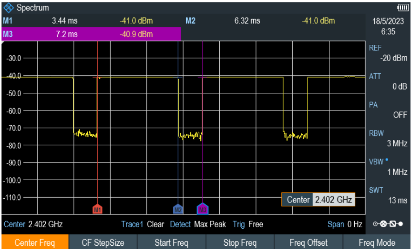
Time-domain plot for Bluetooth transmission signal
