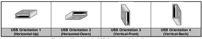
Fig-4.1 Illustration for USB Connector Orientations
