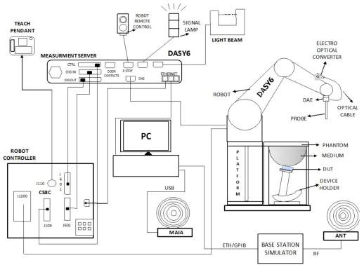
Fig-3.1 SPEAG DASY6 System Setup
