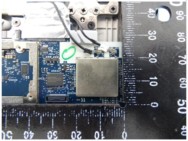
EUT: Wireless Module (Brand Name: HP / Model Name: LBEE58D1VF)
