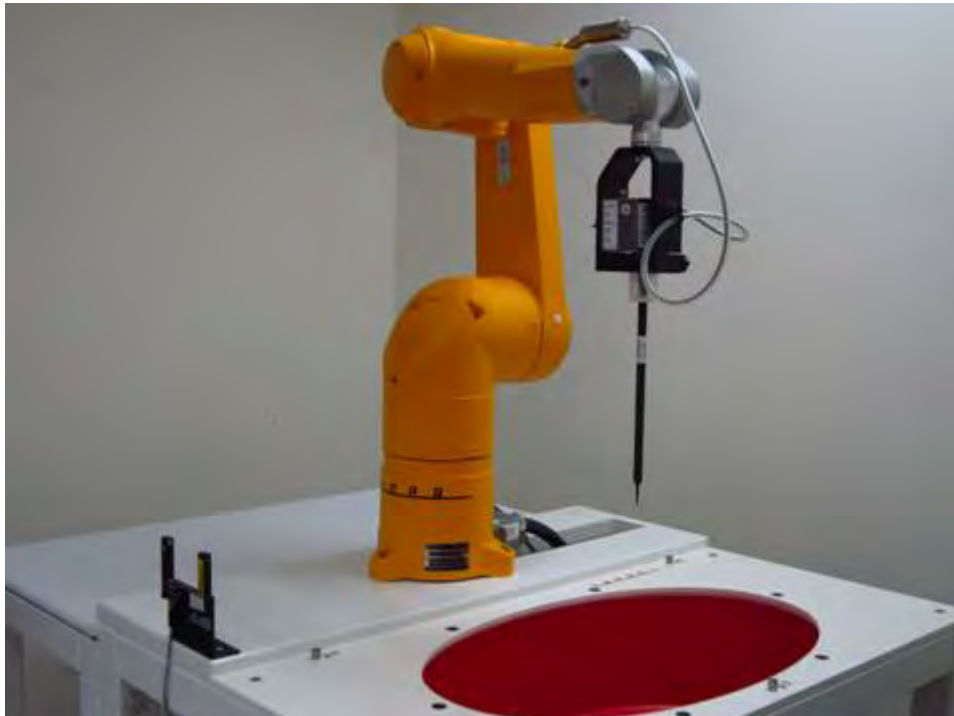
Fig.1 Photograph of the SAR measurement system
