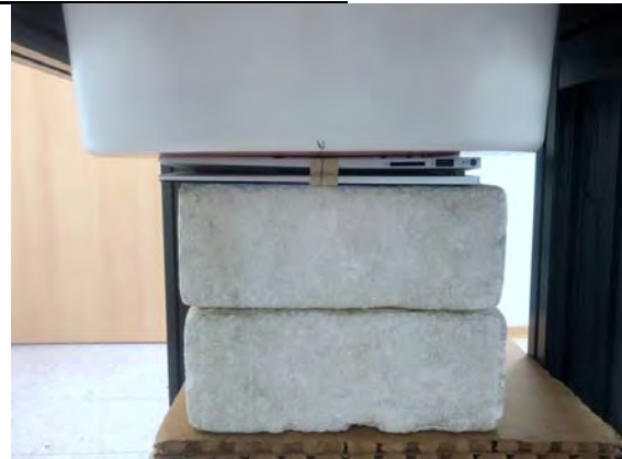
Fig.3 EUT Back side to flat phantom
