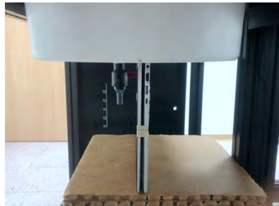
Fig.5 EUT Bottom side to flat phantom
