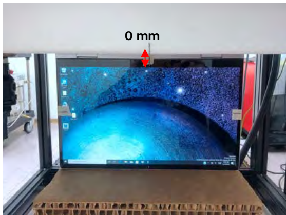
Fig.5 EUT Bottom side to flat phantom
