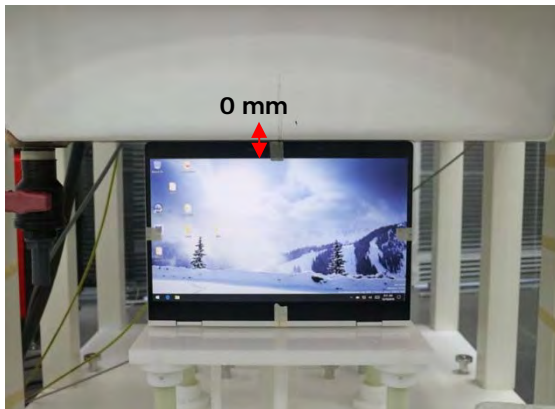
Fig.4 EUT Top side to flat phantom
