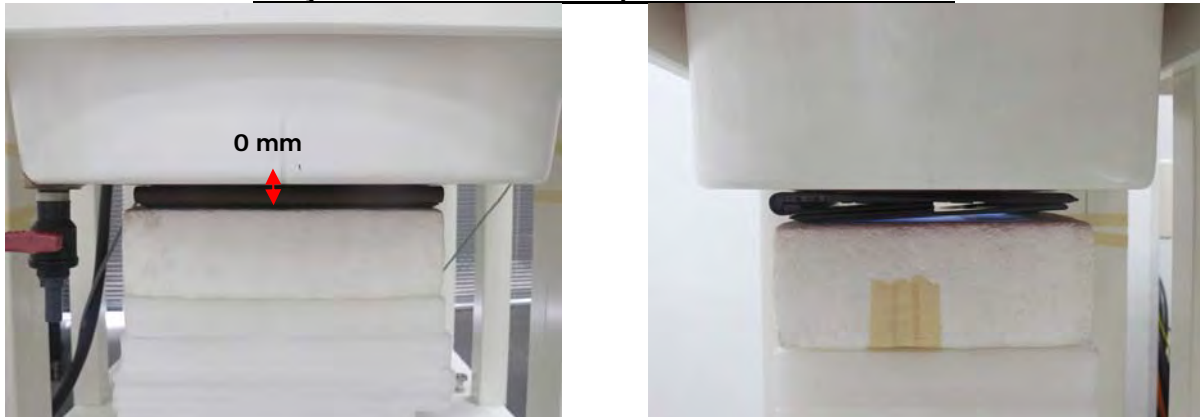
Fig.3 EUT Back side to flat phantom
