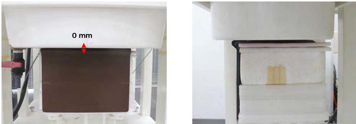
Fig.5 EUT Bottom side (Notebook mode) to flat phantom
