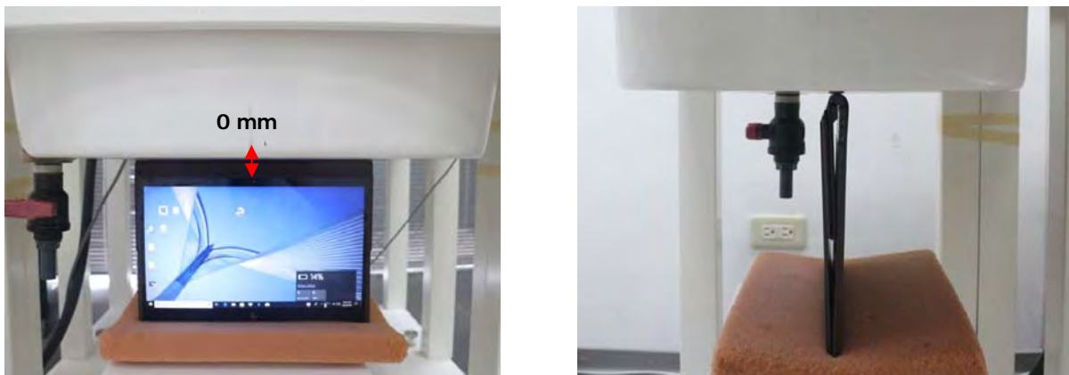
Fig.4 EUT Top side to flat phantom
