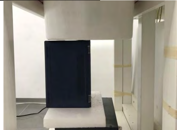
Fig.9 EUT Right side (Book mode) to flat phantom
